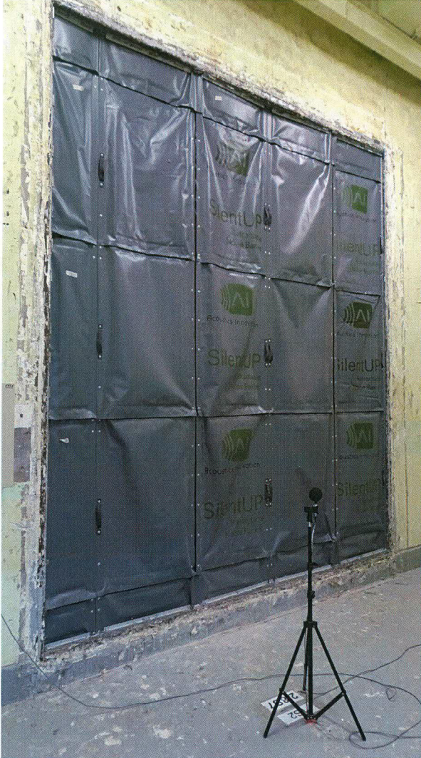
Measurement set-up (Source room)
