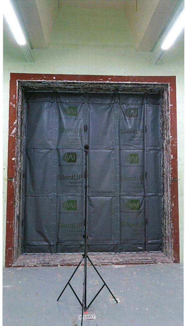
Measurement set-up (Receiving room)
